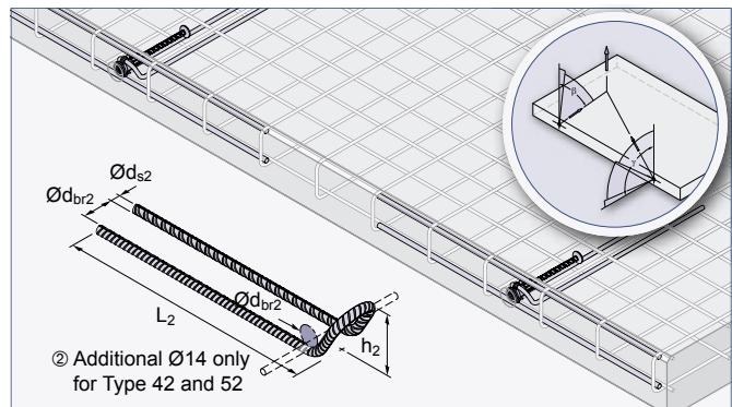
Picture 9 Diagonal and lateral tension - reverse reinforcement for lateral tension
