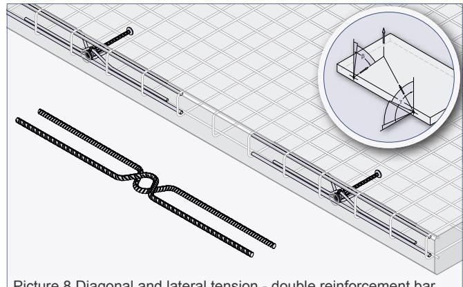
Picture 8 Diagonal and lateral tension - double reinforcement bar
