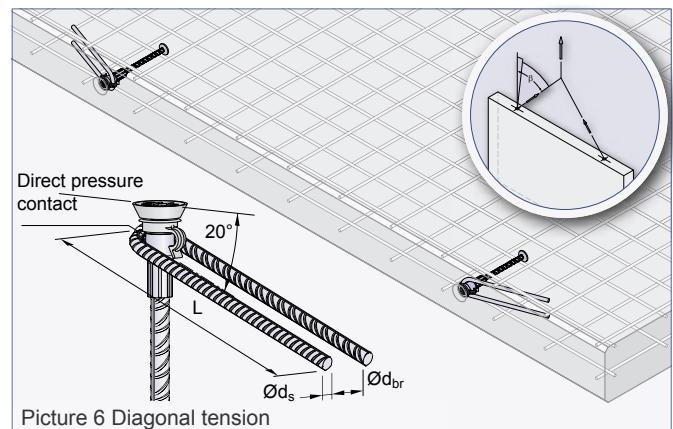
**!** Position of the direct pressure contact between insert and additional reinforcement must be within the thread reach of the insert.
