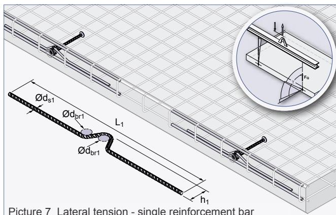
Picture 7 Lateral tension - single reinforcement bar
