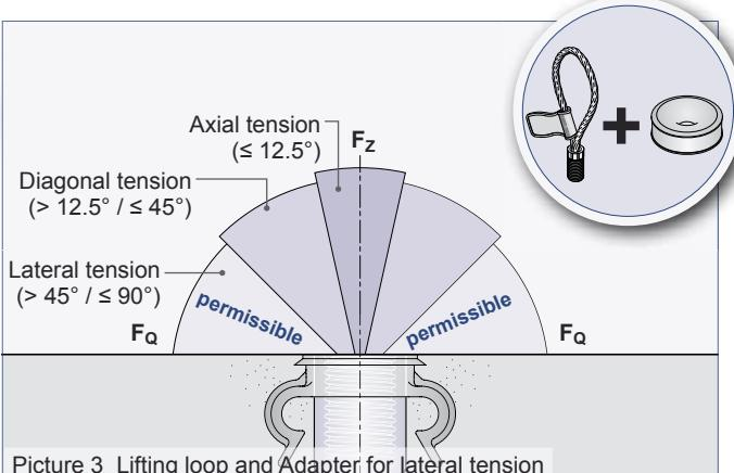
Picture 3 Lifting loop and Adapter for lateral tension
